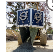
The FlexFold bottom provides controllable material release.
