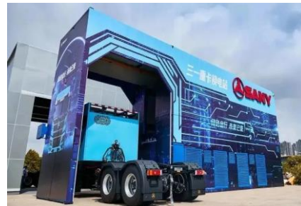
Figur 9, Sany battery swap station
