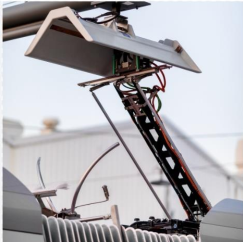
Figure 37 Classical bus charging application using a pantograph.
