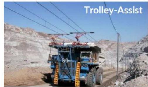
Figure 43 Example of a dynamic charging system (Trolley assist) on rigid dump truck
