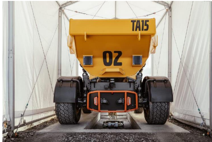
Figure 38 Inverted pantograph charging solution for an autonomous hauler.
